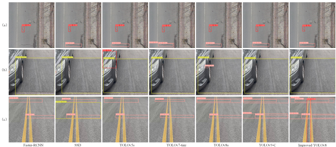
Figure 15. Detection result comparison. (a) Long-distance defective road surface. (b) Short-distance defective road surface. (c) Densely distributed defective road surface.
